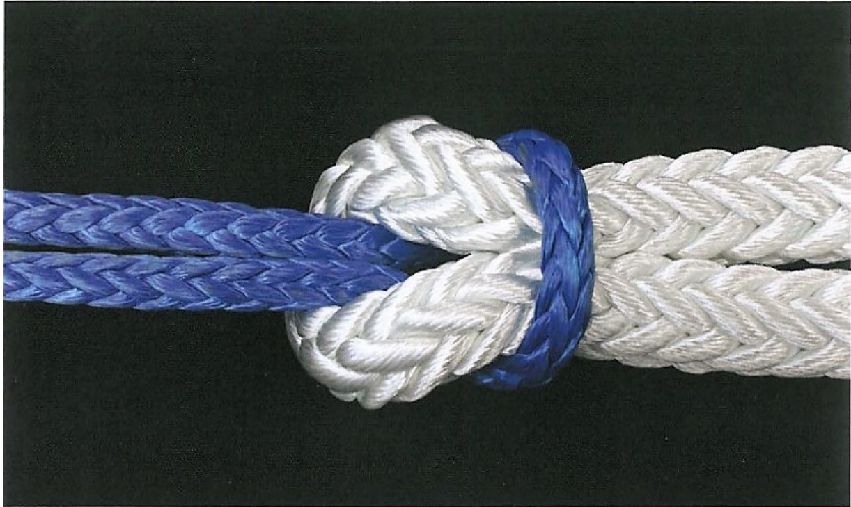
Figure 5.21: Cow hitch connection - HMSF line to polyester tail
