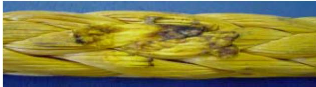
FIGURE D12: ACTUAL MELTING DAMAGE, OFTEN BLACK HARDENED YARN END THAT CAN NOT BE FLEXED BACK. IN THIS PICTURE APPROX. 50% OF ONE STRAND IS ACTUALLY MELTED AWAY.
